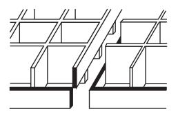
Interlocking step trim design permits panels to be butted together without noticeable joint - providing an uniterrupted louver pattern. This method is accomplished without having to reverse louver panels.
