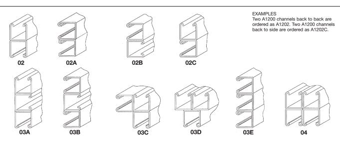
Back to back steel channel is riveted at every 4 inches. Aluminum back to back channel are extruded profiles. All other combinations are spot welded at every 4 inches.
