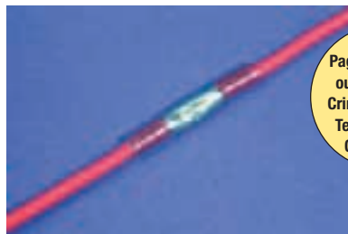
5. Completed Waterproof Connection
