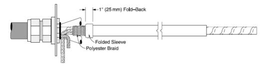
$3M^{TM}$  Cold Shrink QT-III Silicone Rubber Three-Conductor Cable Termination Kits, 7600-3-RJS
