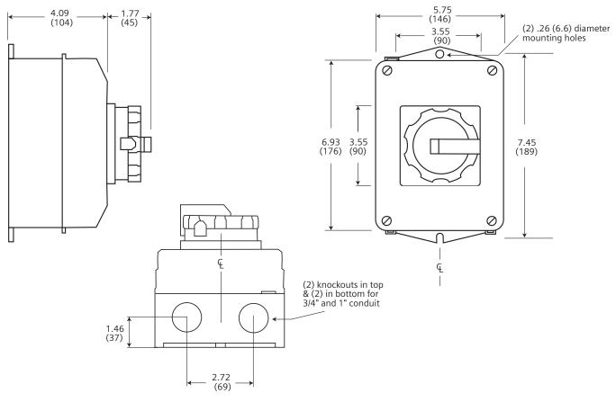
Dimensions shown in inches and millimeters ( ). Dimension shown accurate to  $\pm~1/16$  inch.
