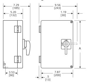
No knockouts in enclosures. Dimensions shown in inches and millimeters [ ]. Dimension shown accurate to  $\pm\,1\%$  inch.
