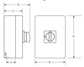
No knockouts in enclosures. Dimensions shown in inches and millimeters ( ). Dimension shown accurate to  $\pm\,1\!\!/\!_{2}$  inch.
