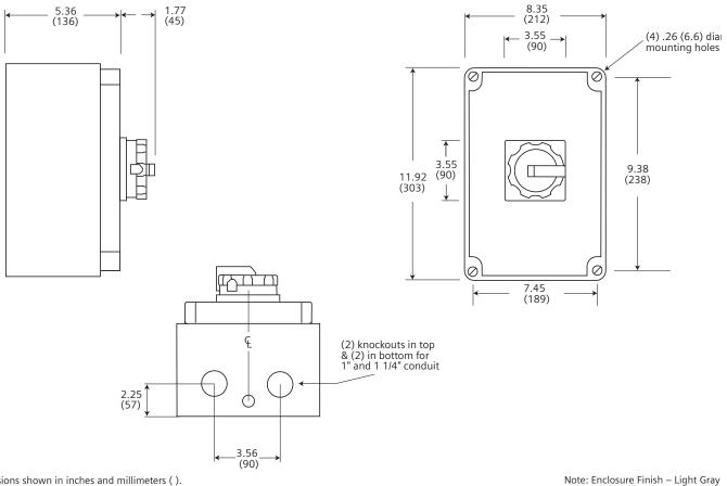
Dimensions shown in inches and millimeters ( ). Dimension shown accurate to  $\pm~1/16$  inch.
