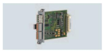
The TB30 Terminal Board supports the addition of digital inputs/digital outputs and analog inputs/analog outputs to the CU320 and SIMOTION D Control Units.
