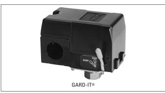
GARD-IT switches are wired in series with a conventional Furnas Brand pressure switch. When failure of the water or air supply causes system pressure to fall considerably below the cut-in point of the regular pressure switch, GARD-IT will turn off the pump motor. When the water supply returns, the system is placed in automatic operation by depressing the manual reset lever until system pressure exceeds the GARD-IT cut off level.
