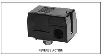
**REVERSE ACTION** pressure switches for air or water cut-in on rising pressure. They are designed to ground the ignition on gas engine driven pumps and compressors when the maximum pressure has been reached, or to act as low pressure alarms, or to prevent pump operation at low pressure. This switch can be supplied with a reset lever.
