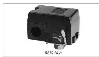
GARD-ALL switches combine the functions of a standard pressure switch with protection against low pressure. They prevent the pump from starting whenever the system pressure falls considerably below cut-in pressure. Upon restoration of the water supply, a manual reset lever is depressed until a build up of system pressure permits automatic operation.
