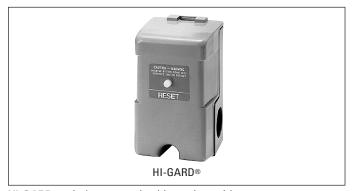
HI-GARD switches are wired in series with any system pressure switch. This special pressure switch is designed to cutout (open the contacts) when a preset pressure is reached and must be manually reset. HI-GARD pressure switch is used when it is desirable to limit the maximum pressure in a system.
