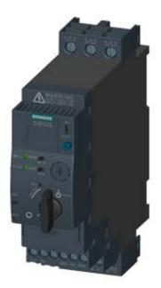
SIRIUS, COMPACT STARTER, DIRECT STARTER 690 V, 110 ... 240 V AC/DC, 50 ... 60 HZ, 1 ... 4 A, IP20, CONNECTION MAIN CIRCUIT: SCREW TERMINAL, CONNECTION AUXILIARY CIRCUIT: SCREW TERMINAL
