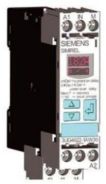
DIGITAL MONITORING RELAY CURRENT MONITORING, 22.5MM FROM 0.05 TO 10A AC/DC OVERSHOOT AND UNDERSHOOT SUPPLY VOLTAGE: AC/DC 24V DC AND AC 50 TO 60 HZ NO GALVANIC ISOLATION FROM MEASURING CIRCUIT STARTUP AND INTERF. PEAK DELAY 0.1 TO 20S HYSTERESIS 0.01 TO 5A 1 CO CONTACT W. OR W/O ERROR LOG SCREW TERMINAL REPLACEMENT PRODUCT FOR 3UG3522-1AC...
