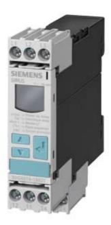
DIGITAL MONITORING RELAY UNBALANCE 0-20% REVERSIBLE PHASE SEQUENCE PHASE FAILURE 3X 160 TO 690V AC 50 TO 60 HZ UNDERVOLTAGE 160-690V HYSTERESIS 1-20V ON AND OFF DELAY 0-20S 2 CHANGEOVER CONTACTS SCREW TERMINAL REPLACEMENT PRODUCT FOR 3UG3012-1A...
