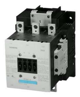
CONTACTOR, 75KW/400V/AC-3, AC(40...60HZ)/DC OPERATION UC 110...127V AUXIL. CONTACTS 2NO+2NC 3-POLE, SIZE S6 BAR CONNECTIONS CONVENTIONAL OPERATING MECHAN. SCREW TERMINAL
