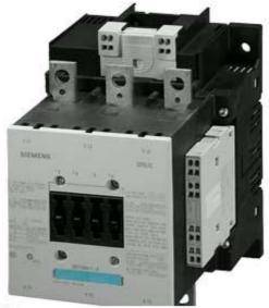
CONTACTOR, 75KW/400V/AC-3 AC(40...60HZ)/DC OPERATION UC 23-26V AUXILIARY CONTACTS 2NO+2NC 3-POLE, SIZE S6 BAR CONNECTIONS CONVENTIONAL OPERATING MECHAN. CAGE CLAMP CONNECTION
