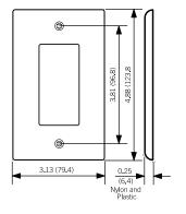
Midway wallplates can be mounted onto larger-volume outlet boxes and/or used to hide wall irregularities. Midway wallplates are a full 0.375" higher and wider than standard size wallplates.
