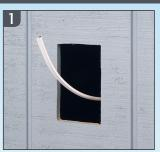
Cut a 3-1/4" x 5-1/2" hole in substrate. Pull wiring.
