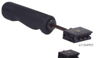
This termination tool is designed to seat 6-110/4-pair connecting blocks and terminate/cut UTP cable on 6-110 wiring blocks.
