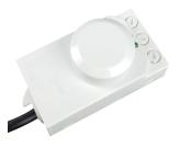
The MS-HF uses high frequency waves to detect motion. The sensor sends out waves that bounce off nearby surfaces and return to the sensor. Motion changes the speed of the waves returning to the sensor. The sensor detects the change in speed and interprets it as occupancy which causes the light to turn on. It triggers primarily through movement of people, objects, machinery. The band of frequency that it usually operates in is <10 mW (about 10x lower than mobile phones)
