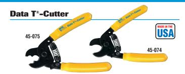
Cuts round communication cable and maintains cable geometry for better cable performance. Data T<sup>®</sup>-Cutter cuts multi-pair cable up to .500 in. (12.7 mm) and coaxial cable up to RG-9/U. Blade cutting capabilities suitable for soft cables (not ACSR).
