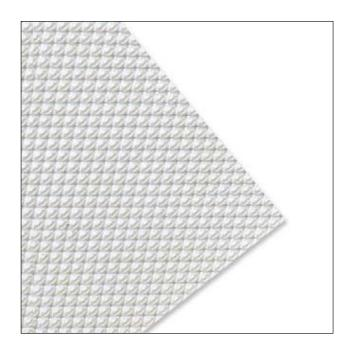
K12 is a quality extruded lens with a square base female conical prism pattern that yields excellent light output and very good brightness control. The diagonally oriented prism pattern, with optically designed square inversed prisms make the K12 an exceptionally strong, lightweight sparkling panel that provides excellent light control.
